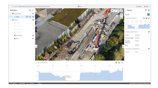
In addition to the distance and area measurements, the platform now offers terrain volume and profile measurement tools. All measurements are performed and displayed in a coordinate and a unit systems selected for the project. For the purposes of tracking changes over time a side-by-side comparison tool has been introduced.
